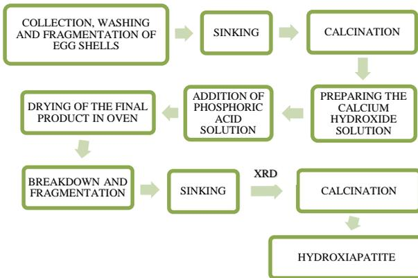
Figure 3. Flowchart showing the obtaining and characterization of hydroxyapatite.
