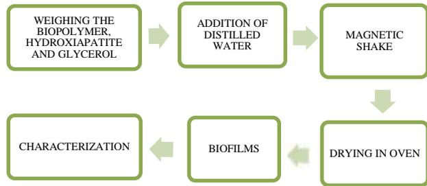
Figure 4. Flowchart showing the production of cassava starch biofilms with hydroxyapatite.
